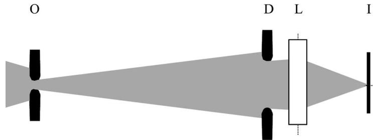
Fig. 1. – Scheme of a focusing system: L is a strong focusing lens which forms the image of the object O at the plane I. The diaphragm D controls the intensity of the beam arriving on the lens L and limits the aberrations introduced by L.
