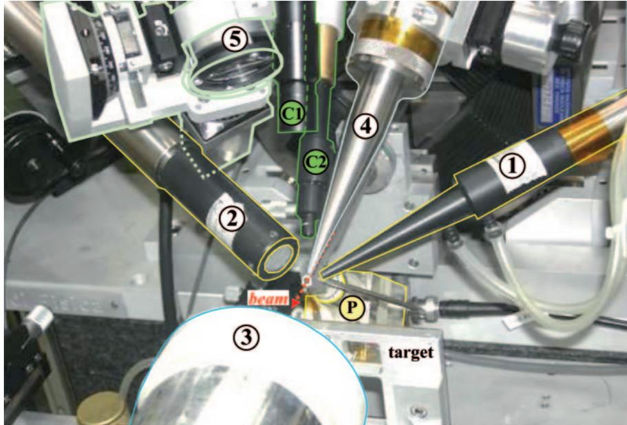
Fig. 3. – Beam end. (1) and (2): X-ray detectors optimized for low-medium- and medium-high-energy X-rays detection (PIXE); (3)  $\gamma$ -ray detector (PIGE); (4) vacuum-tight case containing the Si-photodiode for the detection of particles backscattered by the target (BS); (5) lens for light collection (IL); (P) Si-PIN detector for beam charge measure; (C1) and (C2) cameras for panoramic and microscopic sample visualization.
