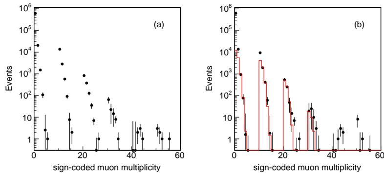
Fig. 5. – Multiplicity distribution of additional muons found in a  $\cos\theta \geq 0.8$  cone around the direction of a primary muon before (a) and after (b) correcting for the fake muon contribution. An additional muon increases the multiplicity by 1 when it has opposite and by 10 when it has same sign charge as the initial muon. The solid line is the prediction of the toy-simulation of a decay into eight  $\tau$ -leptons (see text).
