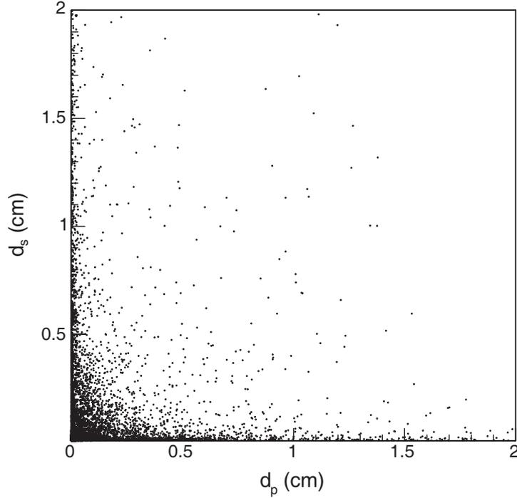
Fig. 3. – Two-dimensional distribution of the impact parameter of an initial muon,  $d_{0p}$ , versus that,  $d_{0s}$ , of additional muons in ghost events. Muons are selected with standard SVX requirements.
