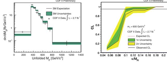
Fig. 6. – Left: differential top pair production cross-section measured by CDF in  $2.7 \text{ fb}^{-1}$  of data using the semileptonic decay mode. Indicated are the total uncertainties for each bin, excluding the overall luminosity uncertainty of 6%. Right: expected and observed limit on  $\kappa/M_{\text{Pl}}$  in a RS model [31, 34].
