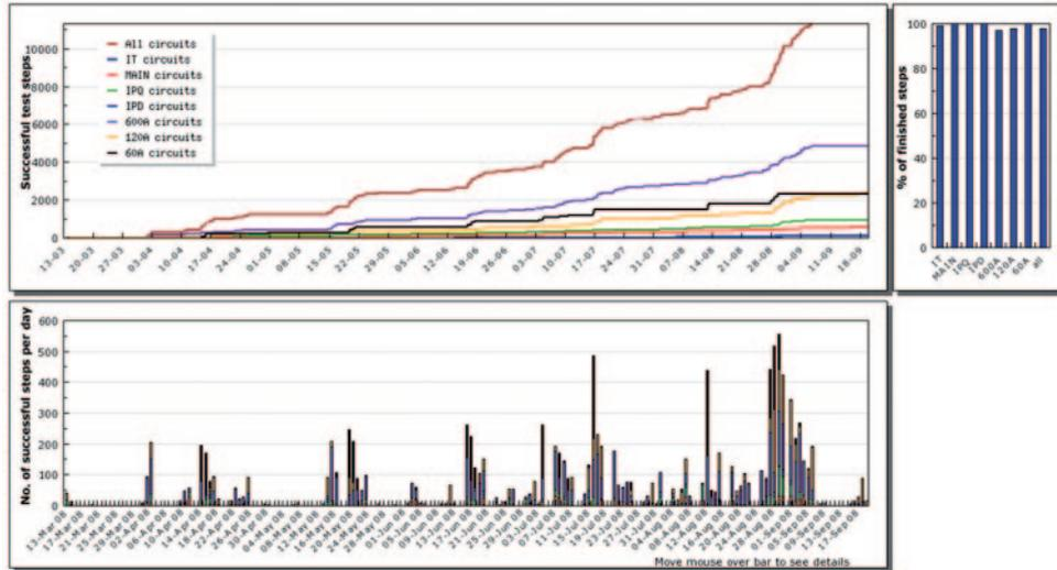
Fig. 1. – LHC Machine Commissioning during 2008: 11122 tests steps completed and successfully achieved (for a total of 11321 to be finally executed).
