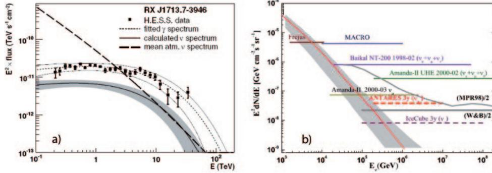
Fig. 1. – (a) Measured gamma-ray flux from the shell-type supernova RX J1713.7-3946 and estimated neutrino flux [3] with their error bands. (b) Sensitivities and upper limits for a  $E^{-2}$  diffuse HE neutrino flux. Experimental upper limits are indicated as solid lines, the ANTARES and IceCube 90% CL sensitivities with dashed lines. For reference, the W&B and MPR98 limits for transparent sources are also shown. Part of the MPR98 upper bound is already excluded by the AMANDA-II result.
