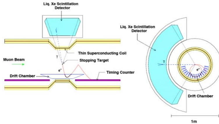
Fig. 1. – Schematic cross-section of the MEG apparatus. A muon beam entering from the left stops in a thin target. The  $\mu^+ \rightarrow e^+\gamma$  decay is detected in a liquid-xenon calorimeter, a set of radial drift chambers and a set of timing counters.
