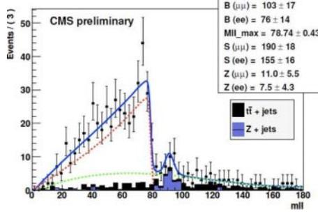
Fig. 3. – Simultaneous fit of the dielectron and dimuon masses (solid line) for  $1 \text{ fb}^{-1}$  of integrated luminosity. On the  $x$ -axis, units are GeV. The signal function (dark dashed line) and the flavour symmetric background function (light dashed line) components are shown superimposed, as extracted from the fit. The lepton cut  $p_T > 20 \text{ GeV}$  was imposed.
