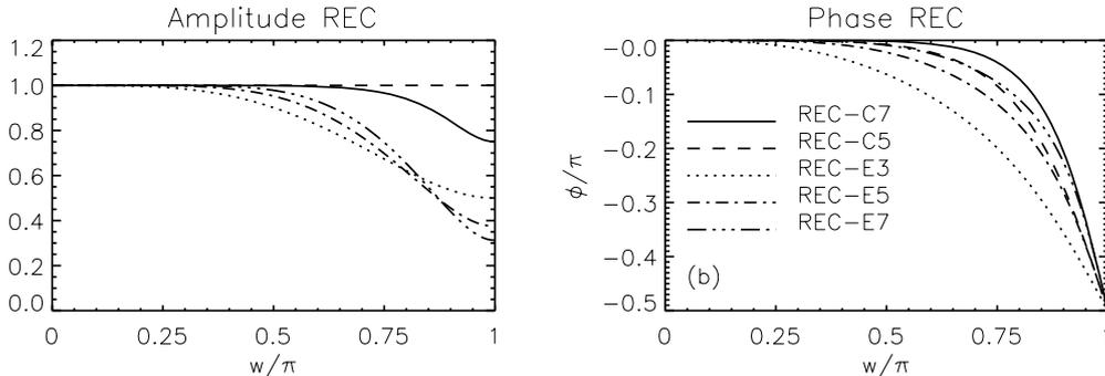
Fig. 1. – Comparison of spectral properties of different high-order explicit and implicit reconstruction procedures. The ideal reconstruction procedure should have unitary amplitude (left panel) and zero phase delay (right) for all values of the normalized wave vector  $w/\pi$ . In the panels are reported the spectral properties for explicit 3rd, 5th and 7th order (E3, E5, and E7) compared to compact 5th and 7th order (C5 and C7).
