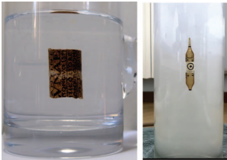
Fig. 1. – A weighted cork (left image) and a cartesian diver (right image) are suspended in a stratified liquid in a cylindrical container. In the case of the diver, the cylinder is sealed on top with a membrane that can be deformed when compressed and transfers the applied pressure to the fluid.
