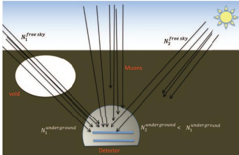
Fig. 1. – Principle of muon radiography by absorption. A detector, placed in an underground tunnel, measures muon flux as a function of direction. The attenuation of the flux depends on the amount of matter traversed by muons. In particular, the presence of a cavity corresponds to an excess of muons.
