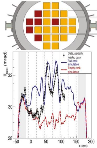
Fig. 5. – Results from the a test on a MC-10 cask, partially filled with fuel assemblies. On the top the sketch of the positions of the fuel assemblies (yellow) and of missing fuel (red). In the bottom the scattering angle measured as a function of the position. The geometrical correspondence of the fuel columns is shown with the dashed lines. Expected result in case of a full and an empty cask are shown as well. Pictures from [11].
