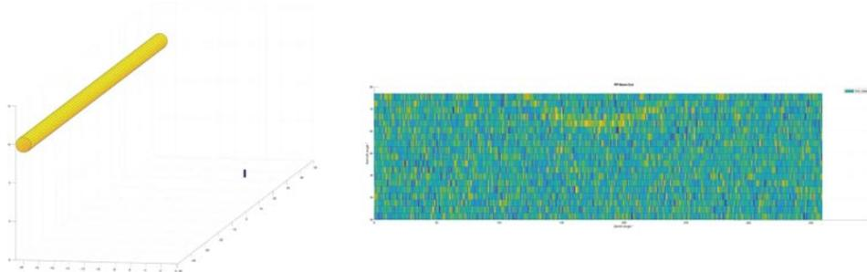
Fig. 3. – Left: the model of a tunnel of 100 m length, 2 m in diameter and located at a depth of 5 m. The borehole detector is placed at a depth of 15 m and at a lateral distance of 20 m. Right; the expected relative transmission after 20 days of data acquisition. The yellow arc shape at the top angular region is the signature of the tunnel.
