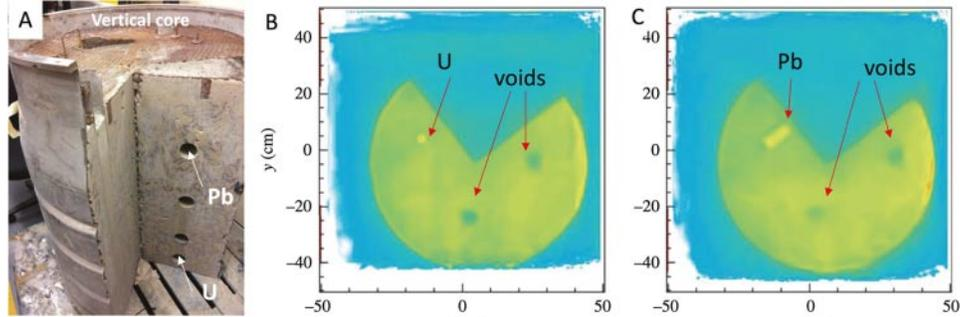
Fig. 7. – (A) The surrogate drum with a 20 mm-diameter, 30 mm-long cylinder of uranium and a lead pieces, measuring approximately 90 mm × 40 mm × 20 mm. (B) and (C): slices of 10 cm thickness obtained of the 3D muon tomography in the region of the uranium (A) and in the region of lead (C). The presence of the two materials as well as the voids are clearly visible. For this analysis 24.7 million muons were collected, for a total acquisition time of about one month. Pictures from [17].
