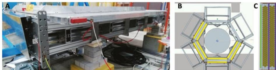
Fig. 6. – (A) Detector segment obtained by adding the INFN Muon Detector (upper part) to the drift tube module (lower part). (B) Detector positions. (C) Top view drawing of a six-layer drift tube muon detector module. Pictures from [15].
