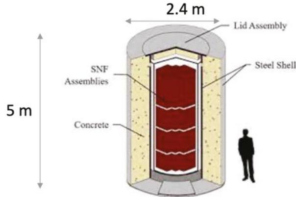
Fig. 4. – A sketch of a typical dry storage cask (DSC). Picture from [5].
