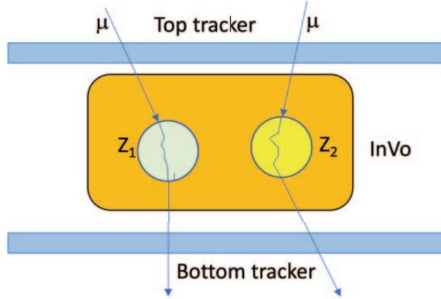
Fig. 2. – Principle of muon radiography by multiple scattering. Two detectors, placed below and above the investigated volume, respectively, measure the entry and exit directions of muons. High-Z material ( $Z_2$ ) tends to scatter muons more than low-Z materials ( $Z_1$ ).
