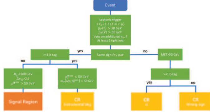
Fig. 2. – Diagram showing the cut-based selection, starting from the event and displaying the requirements for the definition of the SR and the CR for different backgrounds.
