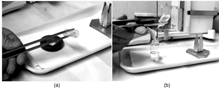
Fig. 8. – Preparation of the point-like (a) and liquid (b) source.
