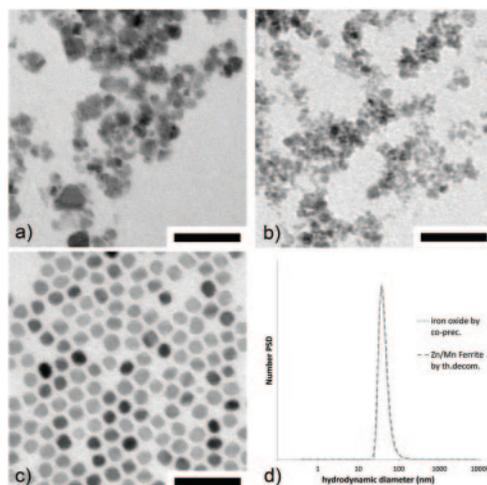
Fig. 1. – TEM images (scale bars of 50 nm) of iron oxide NPs (a) and Zn/Mn ferrite NPs (b) obtained by co-precipitation method and thermal decomposition method (c). In DLS measurement (d), the dashed line represents the Zn/Mn ferrite NPs by thermal decomposition and the dotted line represents the iron oxide by co-precipitation method.
