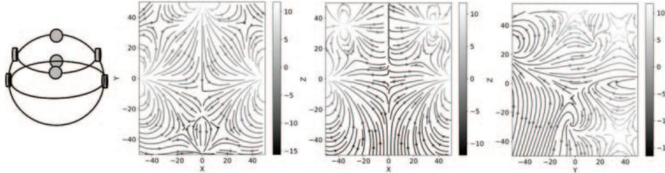
Fig. 2. – Seven magnets ideally located on the wall of a sphere (5 cm radius): three magnets located in the equatorial plane, and four magnets located in a fixed plane at the top of the sphere. Simulations of magnetic fields were performed revealing the direction of magnetic field.
