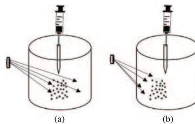
Fig. 1. – A sketch of the setup used to investigate the response of MOLNBs to magnetic fields generated by two different configurations of magnets positioned on the cylinder wall: (a) Four magnets at distance 4 cm each other in symmetric position with respect to the cylinder axis; (b) four magnets positioned in the left side of the cylinder at distance 2 cm each other.
