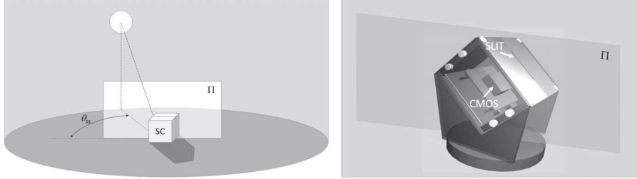
Fig. 1. – Angle \theta_{ss} between the Sun and the solar compass (SC) reference plane \Pi (left). Sketch of the SC, with the slit, the optical sensor (CMOS) and the reference plane \Pi position (right).
