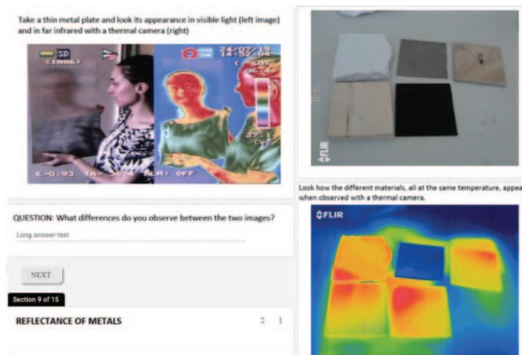
Fig. 1. – Examples of online pages of activity III that aim to introduce students to reflectance and emissivity of matter, starting from the counterintuitive case of metals. On the left, a person close to a metal plate, is shot in visible (left) and far-infrared (right) radiation. In the following form page (right), there is a second set of pictures, which show the visible (top) and thermal (bottom) images of different materials all at the same temperature.
