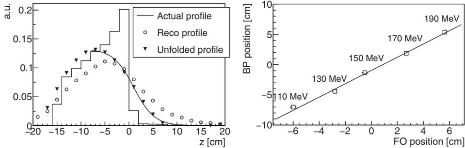
Fig. 2. – Left: normalized profiles of prompt-gamma emission obtained from 160 MeV protons impinging on a PMMA target. The actual production distribution (solid line), the reconstructed profile (circles) and the unfolded profile (triangles) are compared. Right: linear calibration of the Bragg peak (BP) position as a function of the 50% fall-off (FO) coordinate of the unfolded prompt-gamma profile.
