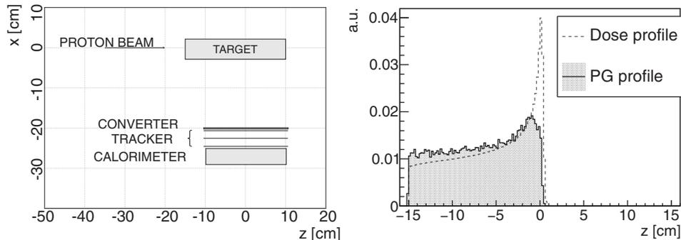
Fig. 1. – Left: visualisation of the simulated FLUKA geometry ( $x$ - $z$  plane view). Right: 160 MeV proton beam dose deposition (dashed line) within the PMMA target, superimposed to the spatial emission distribution of the prompt-gammas (PG) along the beam axis (filled area).
