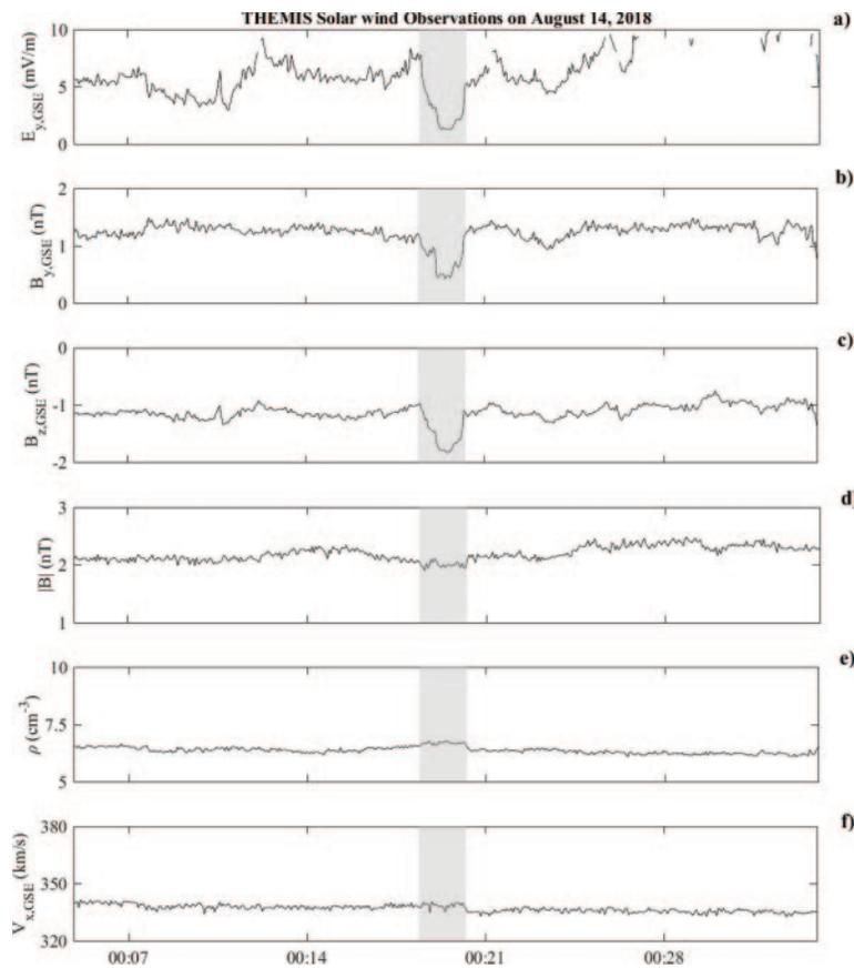
Fig. 2. – THEMIS-C solar wind observations: (a)  $Y_{GSE}$  component of the interplanetary electric field; (b)  $Y_{GSE}$  component of the interplanetary magnetic field; (c)  $Z_{GSE}$  component of the magnetic field; (d) total interplanetary magnetic field; (e) plasma density; (f)  $X_{GSE}$  component of the plasma velocity. All components were expressed in the geocentric-solar-ecliptic (GSE) reference frame.
