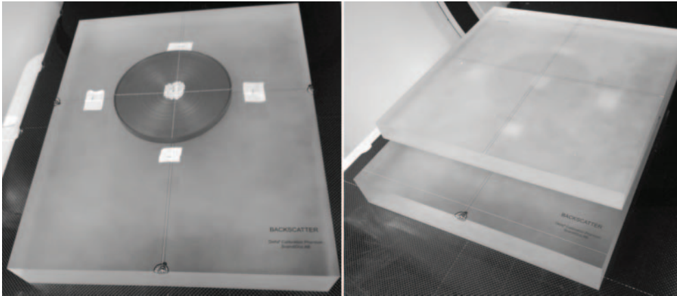
Fig. 1. – Pictures of photon irradiation set-up. Left panel: slab of PMMA phantom with TLDs housed in the water-equivalent disk. Right panel: wafer-like configuration, packaging the disk between 5 cm below and 3 cm above PMMA slab phantom. The lines crossing the center of the disk are the position lasers.
