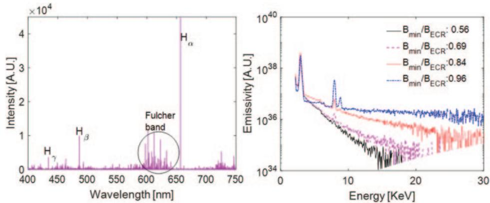
Fig. 3. – On the left, a hydrogen spectrum acquired with a spectropolarimeter with resolution  $R = 16000$ . On the right, typical X-ray spectra emitted by an argon plasma at different magnetic field configurations [35].
