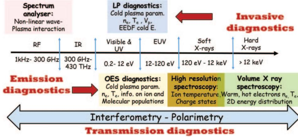
Fig. 1. – Diagnostics methods used for EEDF characterization and related electromagnetic spectrum.
