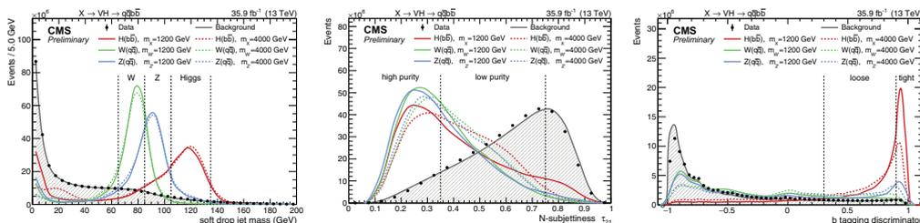
Fig. 1. – Significant variables used to discriminate signal events (coloured curves) with regards to multijet background (in shaded grey): the jet mass (left) defines the signal regions ( $W$  in green,  $Z$  in blue,  $H$  in red);  $\tau_{21}$  subjettiness (center) defines the purity categories for electroweak bosons; the double  $b$ -tagger algorithm outcome (right) defines the categorization when a jet is identified as Higgs boson.
