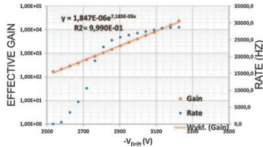
Fig. 1. – Effective gain *vs.* the voltage applied to the drift electrode measured for the GE1/1 detector.
