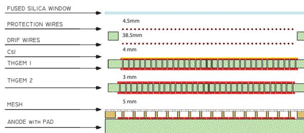
Fig. 1. – Sketch of the hybrid single photon detector. Image not to scale.
