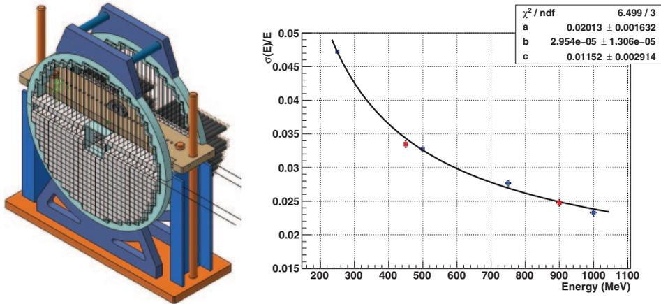
Fig. 5. – Left: design of the PADME calorimeter; Right: measured energy resolution as a function of the deposited energy in the calorimeter prototype [18].
