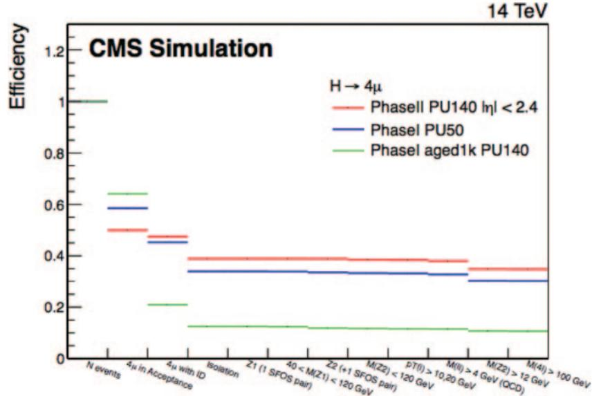
Fig. 4. – Cut flow table showing the event selection efficiency at each step of the analysis for signal  $H \rightarrow ZZ^{(*)} \rightarrow 4\mu$  for Phase-II, reference Phase-I and “aged” configurations.
