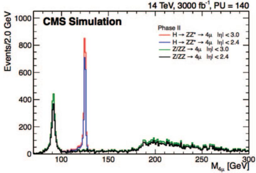
Fig. 7. – Four muons invariant mass distributions for the signal  $H \rightarrow ZZ^{(*)} \rightarrow 4\mu$  and the background  $ZZ \rightarrow 4\mu$  both for the coverage limited to  $|\eta| < 2.4$  and  $|\eta| < 3.0$ .
