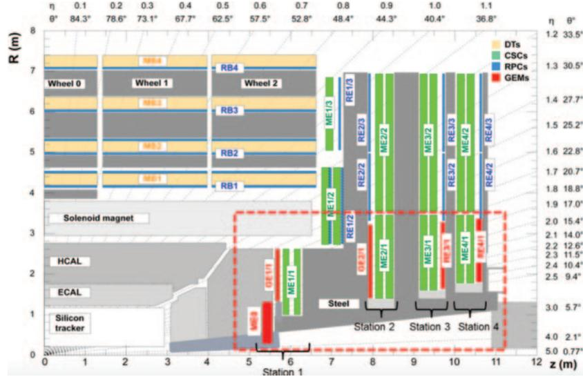
Fig. 2. – Longitudinal view of the CMS detector: planned detector for the muon system upgrades are marked in red.
