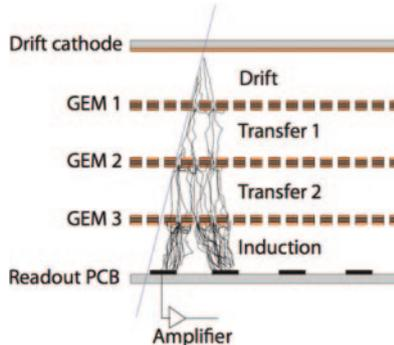
Fig. 3. – Structure of the Triple-GEM detector with three foils, a drift electrode on the top and a read-out electrode at the bottom defining drift and induction fields.
