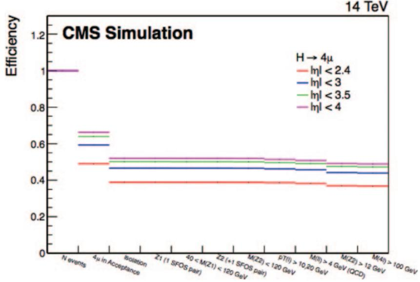
Fig. 6. – Cut flow table showing the event selection efficiency at each step of the analysis for signal  $H \rightarrow ZZ^{(*)} \rightarrow 4\mu$  for Phase-II configuration in different coverage scenarios:  $|\eta| < 2.4$ , 3.0, 3.5, 4.0.
