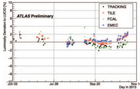
Fig. 1. – Stability of the ATLAS luminometers during the 2015 data taking.
