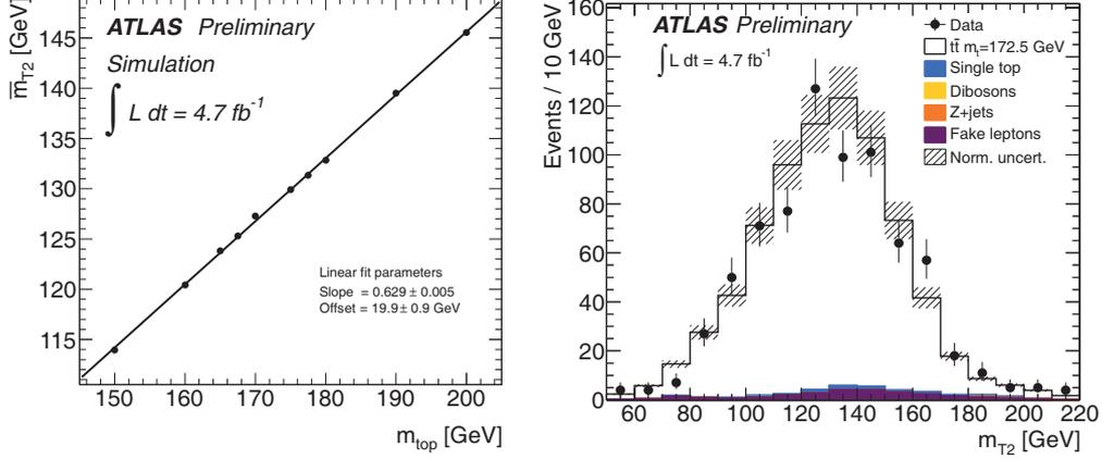
Fig. 1. – The calibration curve (left) determined in MC showing the dependence of the  $m_{T2}$  on  $m_{top}$  and the distribution of the  $m_{T2}$  in MC and data (right) in the dilepton  $e\mu$  channel [4].
