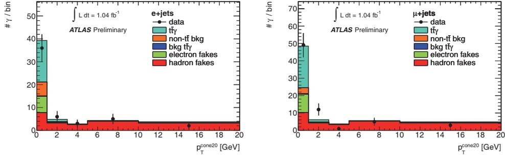
Fig. 4. – The distribution of  $p_T^{\text{cone}20}$  of the photon in the  $t\bar{t}\gamma$  cross section measurement [13]. These distributions are after the template fit in  $e + \text{jets}$  channel (left) and  $\mu + \text{jets}$  channel (right). The predicted  $t\bar{t}\gamma$  signal is shown on top of the different background contributions.
