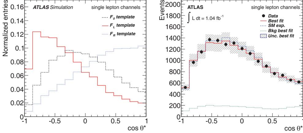
Fig. 5. – The distributions of reconstructed  $\cos \theta^*$  for each of the three simulated signal templates (left) are used for  $W$  helicity measurement [18]. The distributions for data, the Standard Model prediction and the best fit value (right) are shown for lepton + jets channel.
