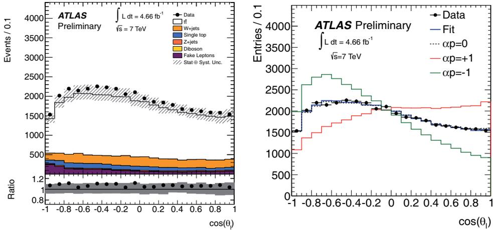
Fig. 2. – The distribution of  $\cos \theta_l$  in data is overlaid with the prediction in MC, where top-quarks in  $t\bar{t}$  production are not polarized (left). A fit is performed using positive and negative polarization top-quark templates (right). Both are for  $\mu +$  jets channel. Corresponding plots for  $e +$  jets channel can also be found in the paper of the top-quark polarization [8].
