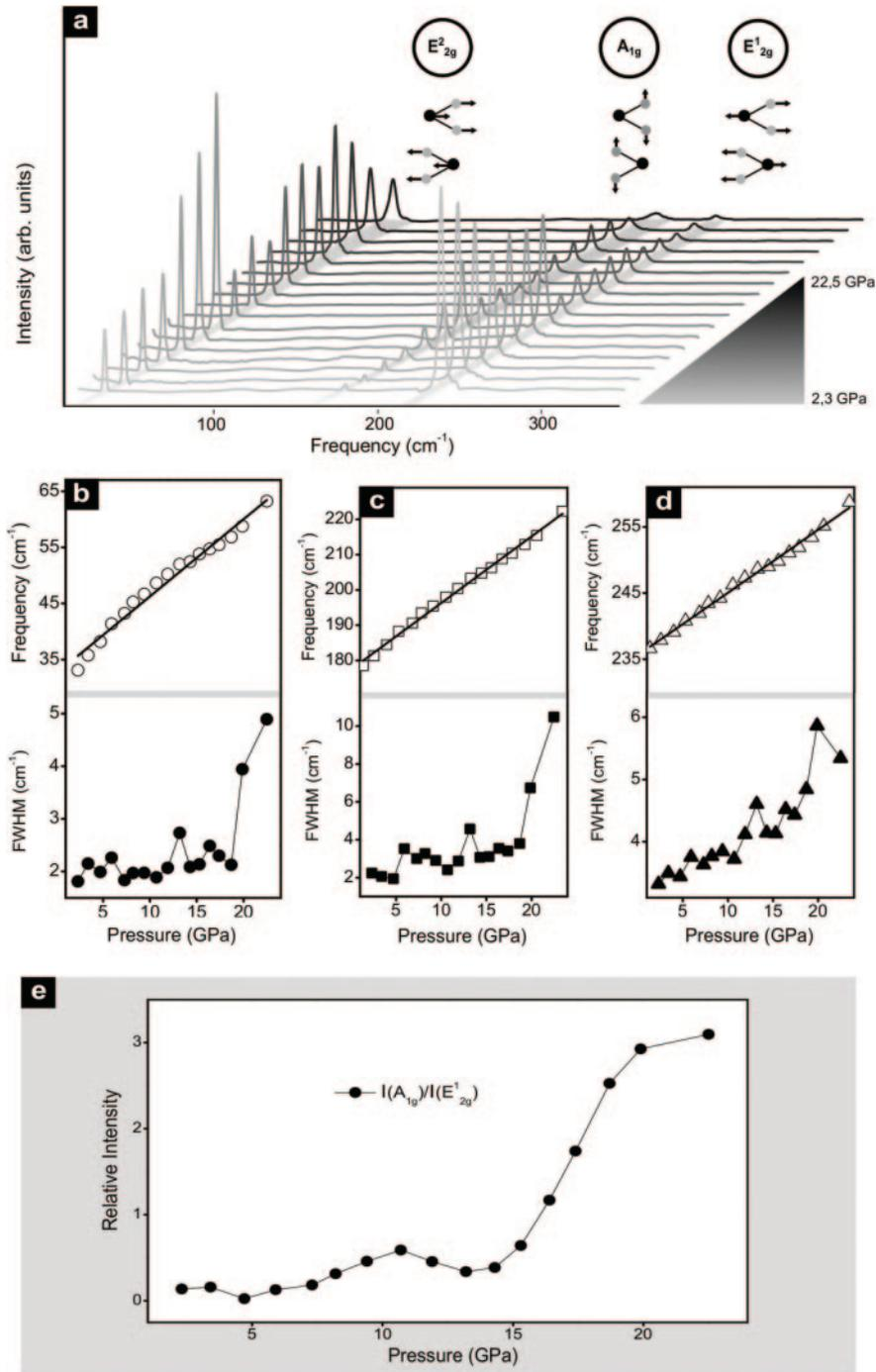
Fig. 1. – Panel (a): MoTe<sub>2</sub> Raman spectra in the range 2–23 GPa. Panels (b), (c), (d): evolution of the peak position and FWHM as a function of the pressure for the  $E_{2g}^2$  (b),  $A_{1g}$  (c),  $E_{2g}^1$  (d) modes. Panel (e): evolution of the relative intensity  $I(A_{1g})/I(E_{2g}^1)$  as a function of the pressure.
